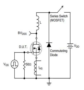
Figure G.Unclamped Inductive Switching Test Circuit
