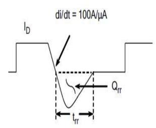
Figure F.Diode Reverse Recovery Waveform
