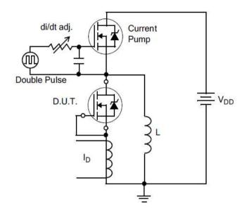
Figure E.Diode Reverse Recovery
