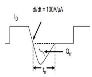
Figure 16. Diode Reverse Recovery Waveform
