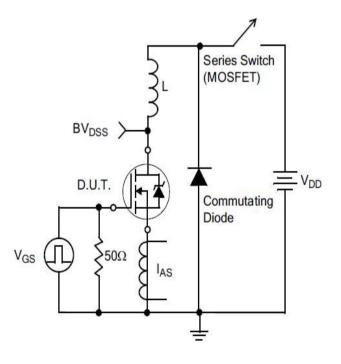
Figure 17. Unclamped Inductive Switching Test Circuit
