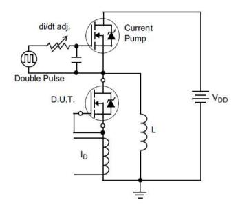
Figure 15. Diode Reverse Recovery
