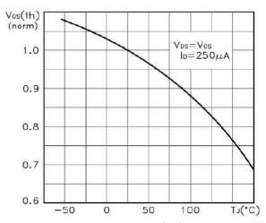
TJ-Junction Temperature ( $^{\circ}$ C) Figure 10 VGS(th) vs Junction Temperature
