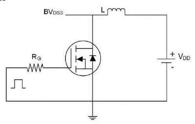
2) Gate charge test Circuit:
