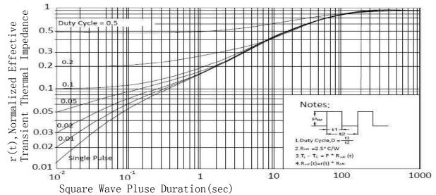
Figure 11 Normalized Maximum Transient Thermal Impedance
