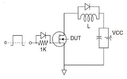
3) Switch Time Test Circuit:
