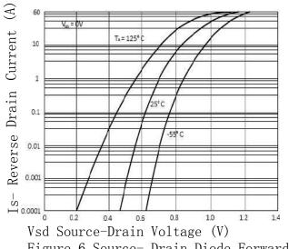
Figure 6 Source- Drain Diode Forward
